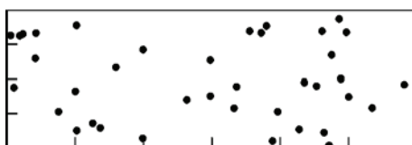
Figure B.4 — A = 2,5\% , d = 1\text{ mm} , 38 pores
