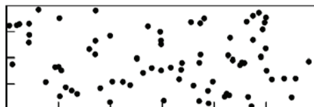
Figure B.7 — A = 5 \% , d = 1 \text{ mm} , 76 pores
