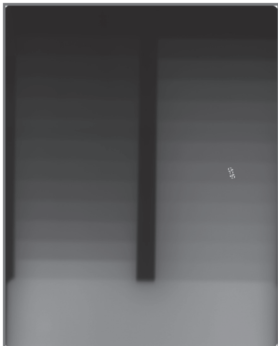
Figure D.2 — Measurement results of mean grey value and SNR_N of a step of the step wedge image
