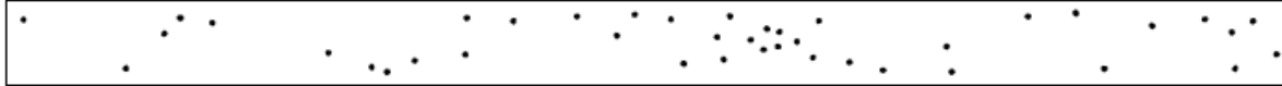
Typical Quantity and Size Permitted in 6 in. (150 mm) Length of Weld 1/8 in. (3 mm) to 1/4 in. (6 mm) Thickness
